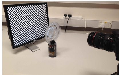
Fig. 19 Real reconstruction setup for thin transparent objects.
