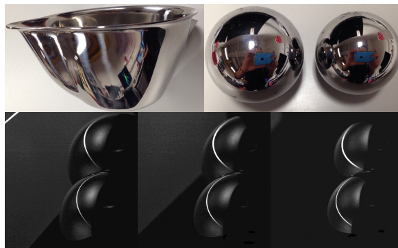
Fig. 3.9 Top row: sauce boat and two spheres in real experiments. Bottom row: a sweeping line is reflected by two spheres under three distinct positions of the LCD monitor while the camera and mirror surfaces are stationary.
