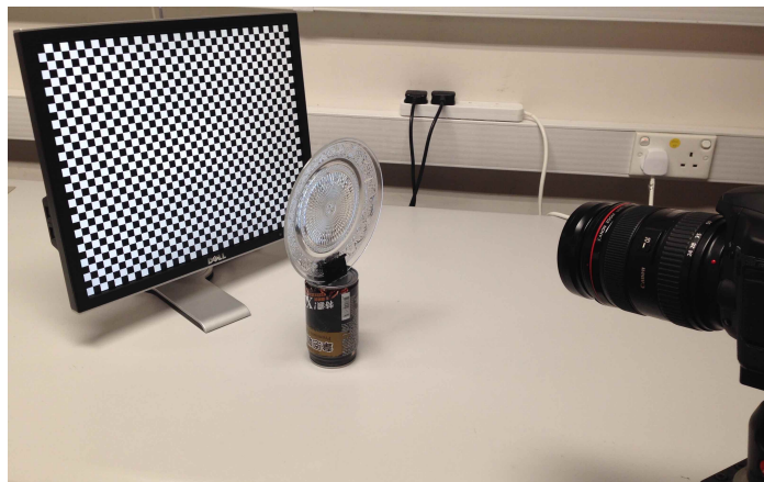
Fig. 2.19 Real reconstruction setup for thin transparent objects.
